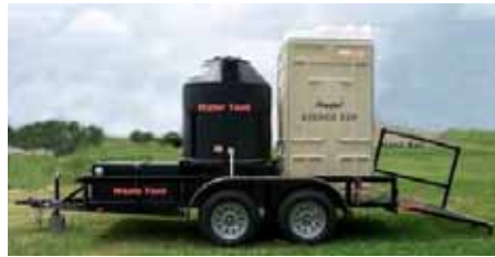
SJSDCS 520 Self Contained Mobile Comfort Station
